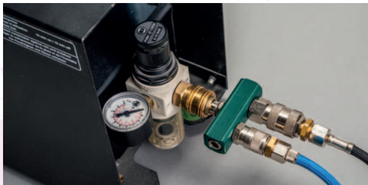
b) If you have a compressor with only one compressed air outlet and you want to connect two airbrushes, you can use a manifold. This example is equipped with two different diameters of 5mm and 7.2mm quick release couplings with 1/4" thread.
