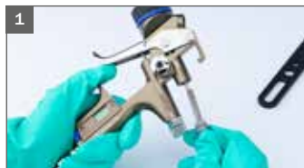
First remove paint needle.
