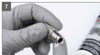
Grease thread of material flow control screw
