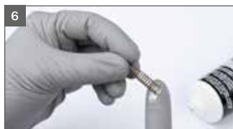
Grease and insert paint needle spring
