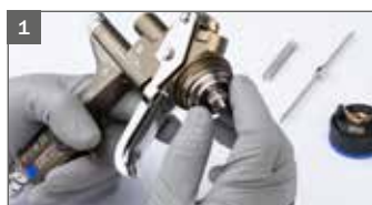
Assembly of the fluid tip
