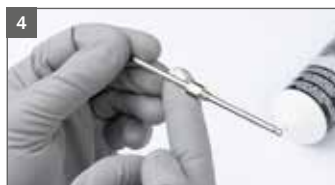
Grease paint needle around the needle packing area
