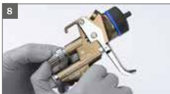
Install material flow control screw
