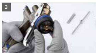
Assembly of the air cap
