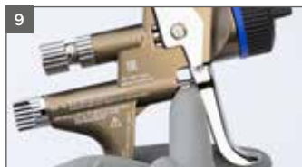
Grease visible part of air piston rod
