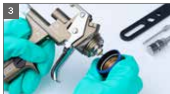
And finally, unscrew fluid tip with the ring spanner integrated in the universal spanner.
