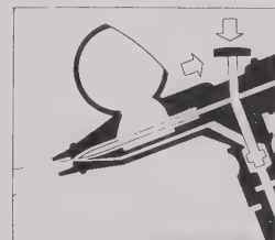
Double-action internal mix
