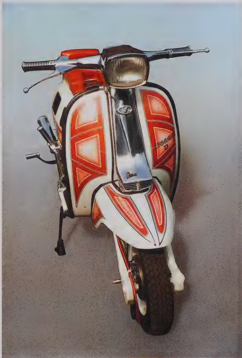
Above: Scooter – showing clever use of narrow masking tape to create a panelled effect that looks more
